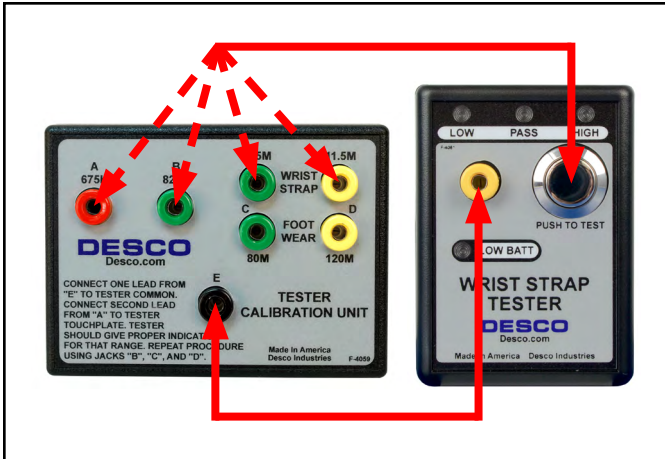
Figure 3. Verifying the calibration of the Wrist Strap Tester
