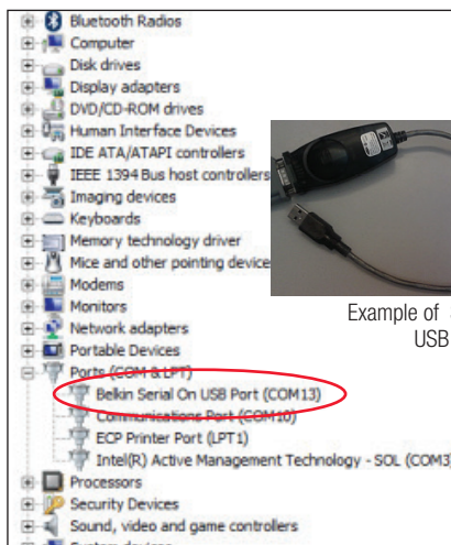
Figure 15: Installation of device appears. In this case, it is of a RS232 Serial to USB adaptor for Port (COM13).
