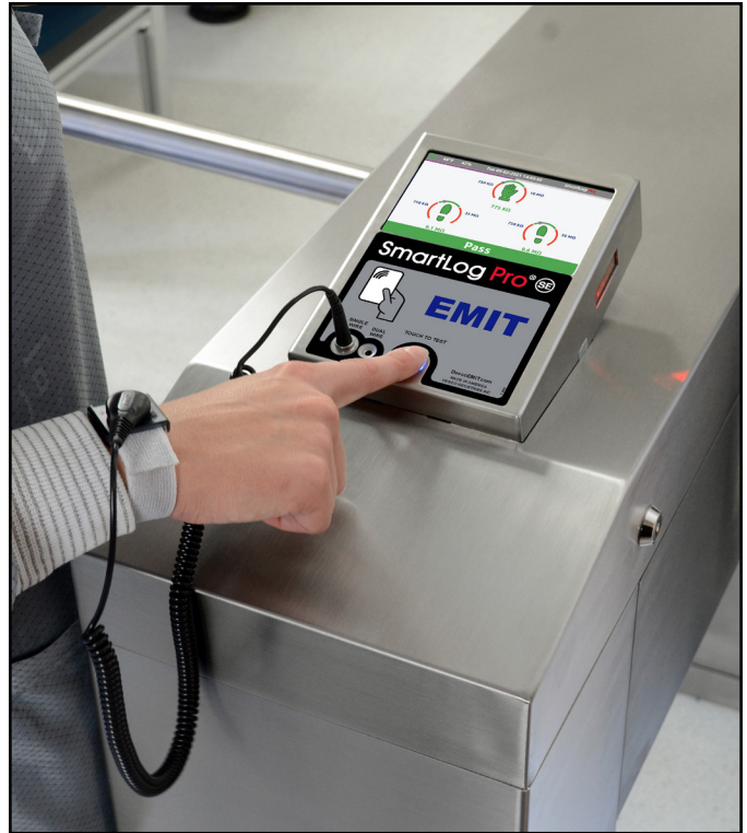
Figure 7. Performing a footwear and wrist strap test
