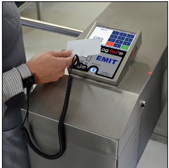
Figure 5. Holding a proximity badge in front of the RFID icon on the SmartLog Pro® SE
