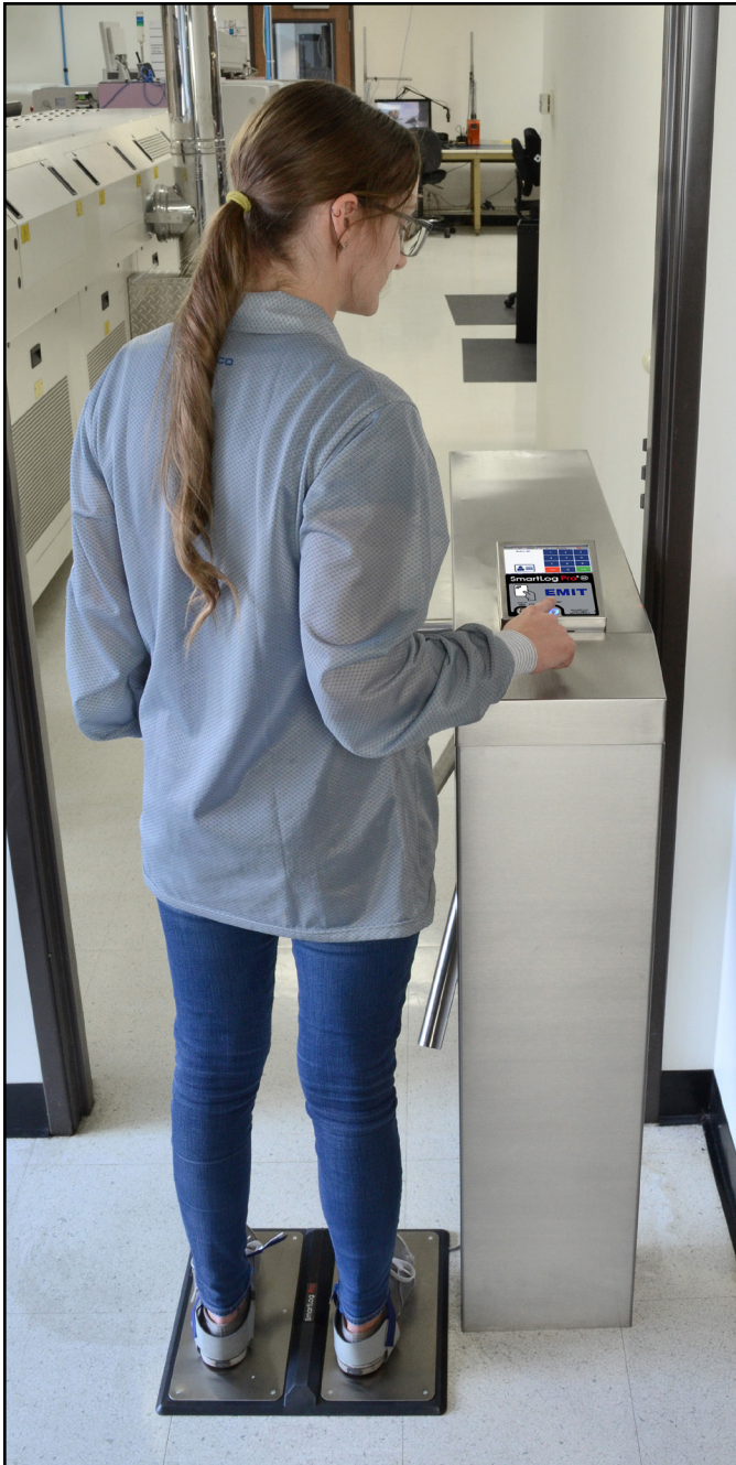
Figure 6. Performing a footwear test
