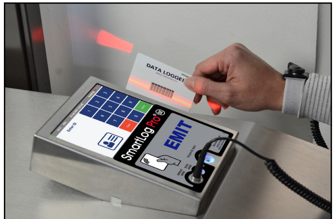
Figure 4. Using the barcode scanner
