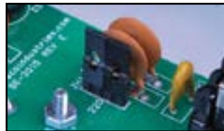
Figure 7. 120 VAC jumper setting
