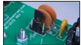
Figure 8. 220 VAC jumper setting
