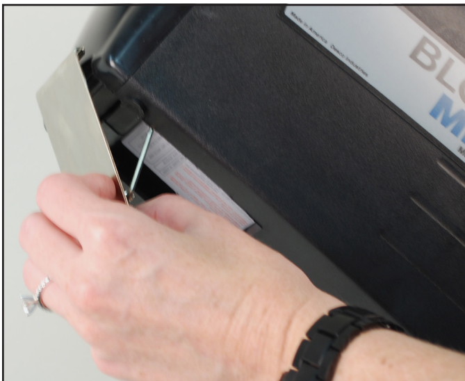
Figure 4. Releasing the filter
