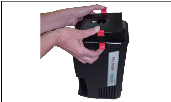
Figure 3: Lifting out the cartridge.
