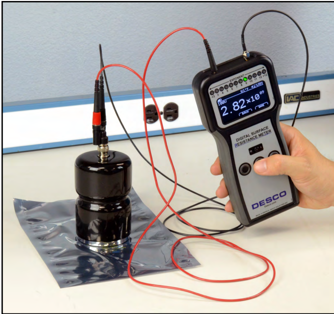
Figure 2. Using the Concentric Ring Probe with the Desco Digital Surface Resistance Meter
