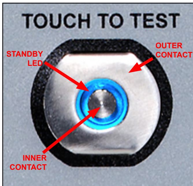
Figure 10. Steady-State Test Switch features and components
