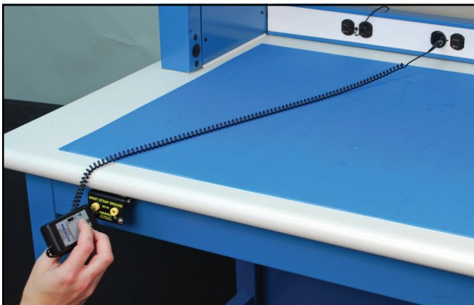
Figure 3. Testing ground points with the 19249 tester
