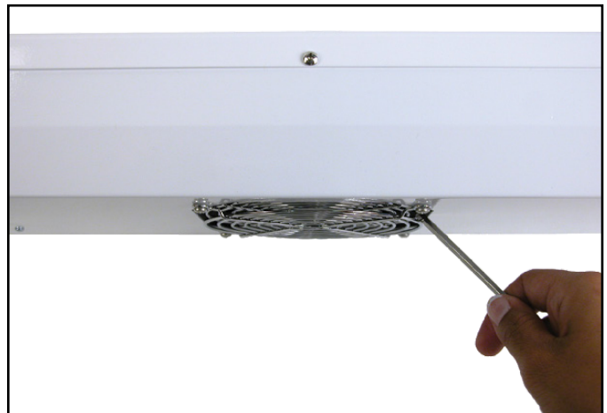
Figure 8. Shorting the ionizer's two fan grills
