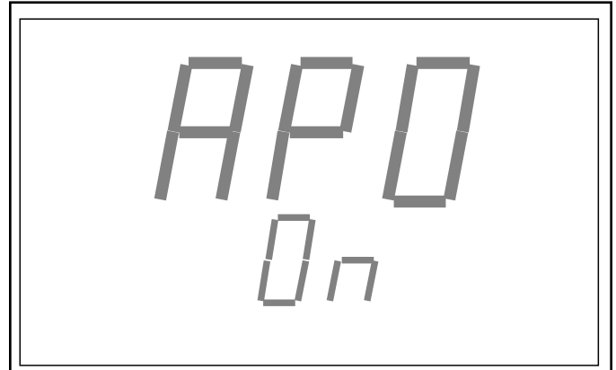
Figure 4. Automatic Power Off (APO) display
