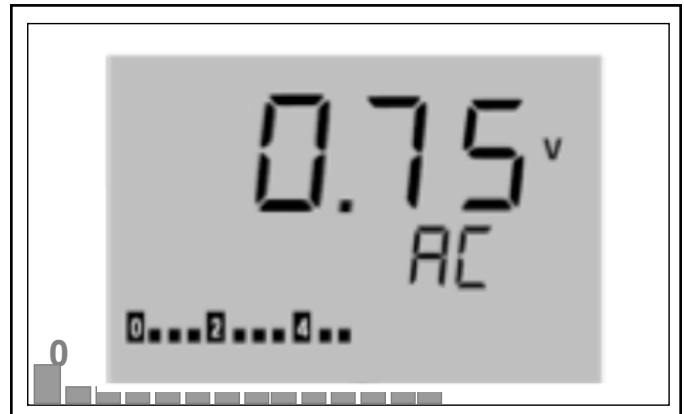
Figure 9. AC voltage display
