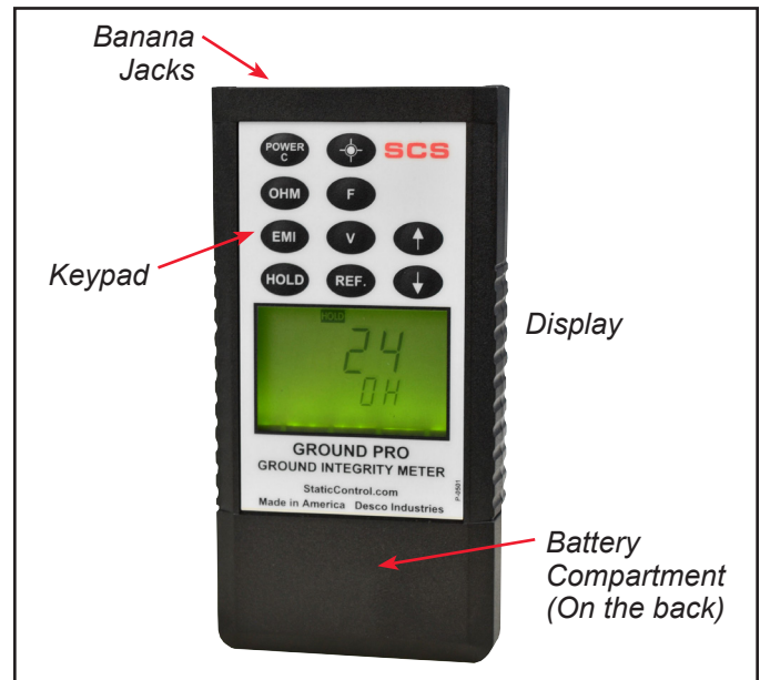
Figure 2. Ground Pro Meter features and components
