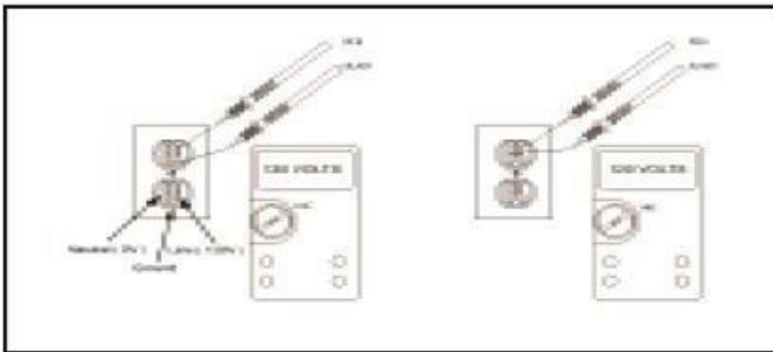
Measure the AC voltage between Ground and the Neutral and the Line respectively.
