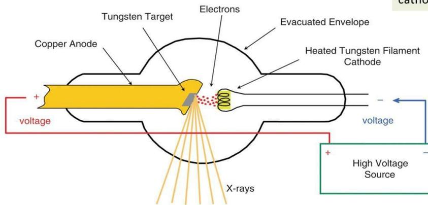
X-ray are only present when power is applied to the x-ray tube
