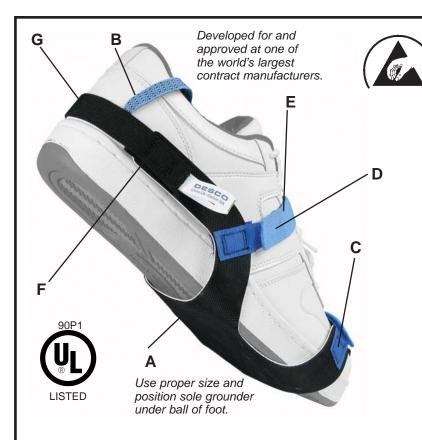
Per ESD SP9.2 APPENDIX B - Foot Grounder Usage Guidance "Compliance verification should be performed prior to each use (daily, shift change, etc.). The accumulation of insulative materials may increase the foot grounder system resistance. If foot grounders are worn outside the ESD protected area testing for functionality before reentry to the ESD protected area should be considered."
