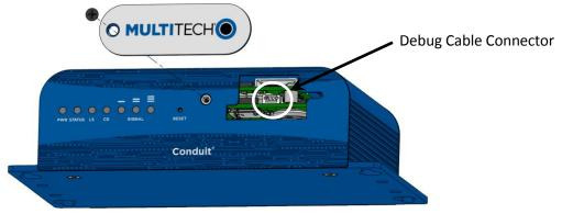
Conduit devices with substitute components will ship with a custom 3-pin cable connector:
