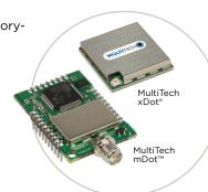
The mDot and xDot are LoRaWAN compliant,
