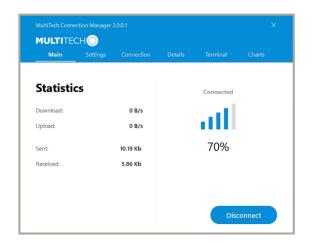
communicate to the Internet whenever needed by ensuring the cellular connection is always ready for transmission, ensuring the smooth operation of real-world IoT use cases. AT Commands, traditionally used to manage these functions, can prove time-consuming and difficult to the un-initiated. Connection Manager provides a much easier and faster method of managing USB and serial cellular modems to ensure persistent connectivity to the cellular network.
