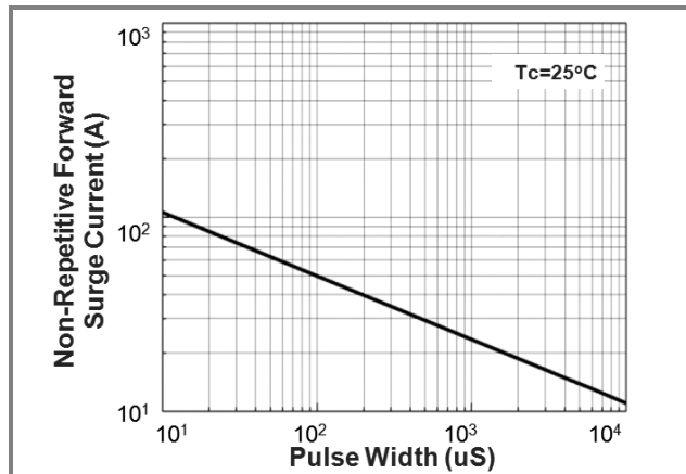
Fig.4 Non-Repetitive Peak Forward Surge Current (Pulse Mode)
