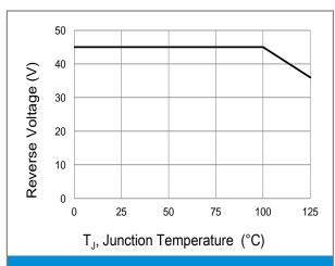
**Fig.4 Operating Temperature Derating Curve**
