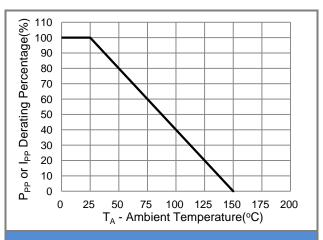
Fig.2 Derating Curve
