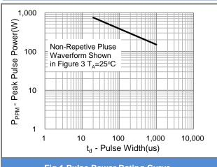
Fig.1 Pulse Power Rating Curve
