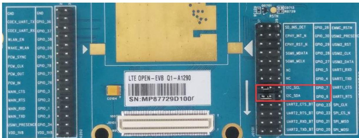
Figure 39: EEPROM Function GPIO Configuration
