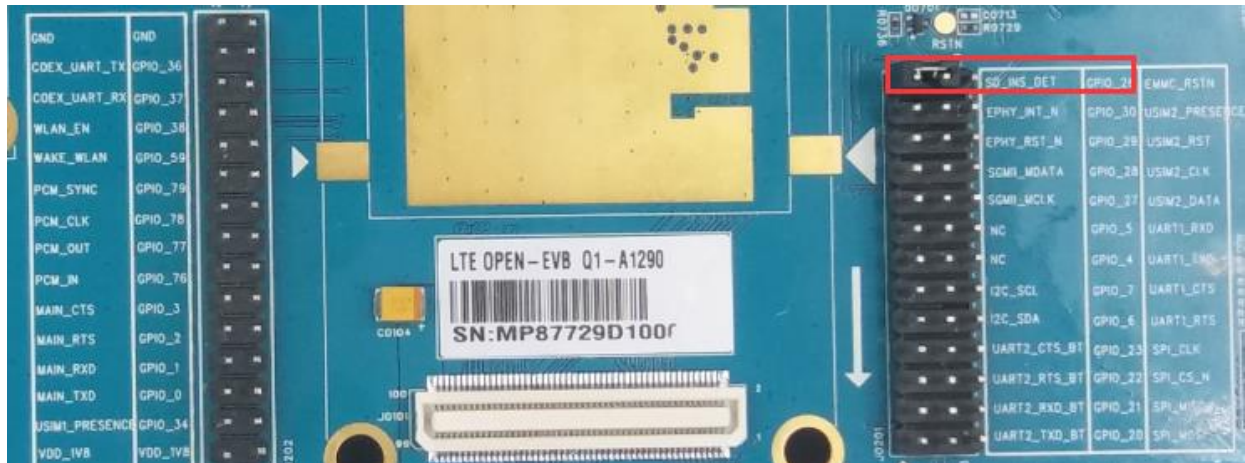
Figure 29: SD Card Function GPIO Configuration
