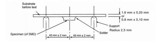
Weld the product to the central part of the PCB with the thickness  $1.6 \pm 0.2$  mm or  $0.8 \pm 0.1$  mm as the illustration shows, and keep exerting force arrow-ward on it at speed of 1 mm/s, and hold for  $5 \pm 1$  seconds at the position of 1.5 mm bending distance, so far, any peeling-off of the product metal coating should not be detected.
