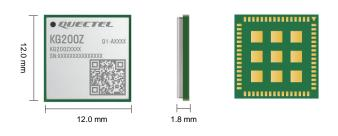
KG200Z is a high-performance LoRa module launched by Quectel, which supports ultra-low power consumption and long-range wireless transmission applications. It integrates an ARM Cortex-M4 core with the modulations of LoRa, (G)FSK, (G)MSK and BPSK, supporting LoRaWAN standard protocol and 470–510 MHz, 862–928 MHz LoRa frequency bands. Additionally, it incorporates AES hardware encryption for enhanced security.
