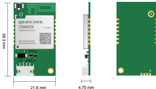
FCMA62N is a cutting-edge MCU Wi-Fi and Bluetooth module launched by Quectel. It boasts a high-performance processor (ARM Cortex-M33) with a frequency of up to 260 MHz and supports IEEE 802.11a/b/g/n/ac/ax protocol and BLE 5.3. The module features built-in 1.2 MB SRAM and 8 MB flash, ensuring efficient performance. In addition, it complies with WPA-PSK, WPA2-PSK, and WPA3-SAE security standards, providing an AES-128 encryption algorithm.
