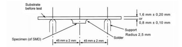
Weld the product to the central part of the PCB with the thickness  $1.6 \pm 0.2$  mm or  $0.8 \pm 0.1$  mm as the illustration shows, and keep exerting force arrow-ward on it at speed of 1 mm/s, and hold for  $5 \pm 1$  s at the position of 1.5 mm bending distance, so far, any peeling-off of the product metal coating should not be detected.
