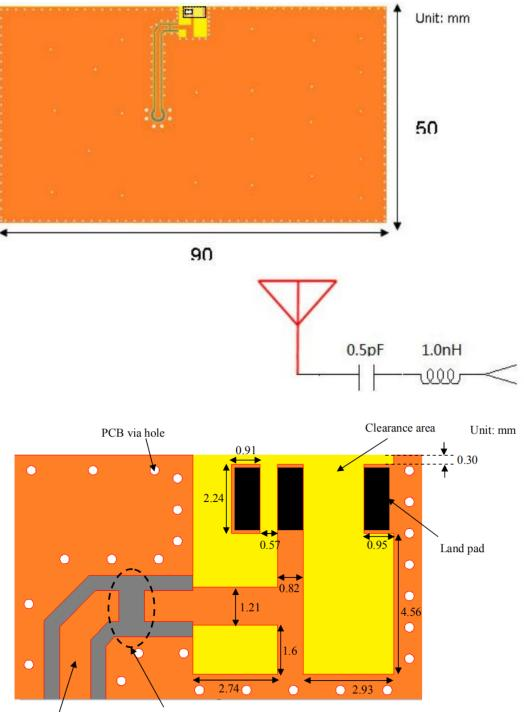
50 ohms feeding line T type matching circuit
