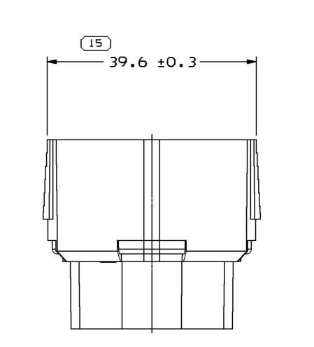
12160280 A7 -M3592025 PA66 HS GRA MD 101 13.295 VOL (CM3) PART NO REV N/P STATUS MATERIAL SPECIFICATION AND COLOR TYPE
