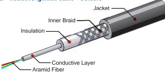
**TYPE 3 – Resistive Ignition Cable – Delcore
