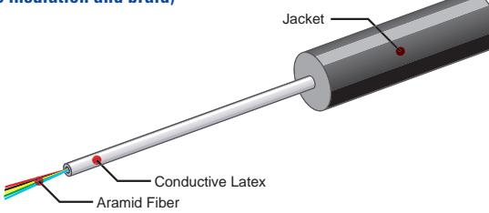
**TYPE 4 – Resistive Ignition Cable – Delcore
