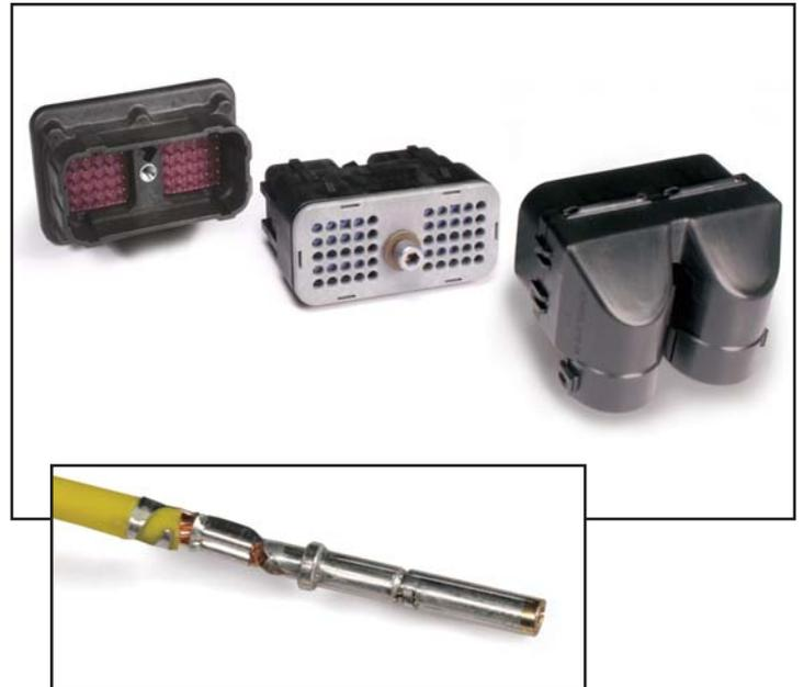
The female connector uses a unique pre-stage feature which aids in ensuring the terminals are fully seated. The harness connector is initially plugged, in the pre-staged position, with the V100 terminals. The connector is closed with the harness build tooling. If a terminal were not fully seated, this secondary connector operation pushes a partially seated terminal into place, virtually eliminating unseated terminals in the vehicle assembly plant.
