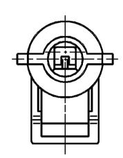
2. MATING CONNECTOR 12089912 OR EQUIVALENT. 3. CONNECTOR TO ACCEPT 12065249 SECONDARY LOCK OR EQUIVALENT. 4. USE 12052834 CONNECTOR POSITION ASSURANCE.
