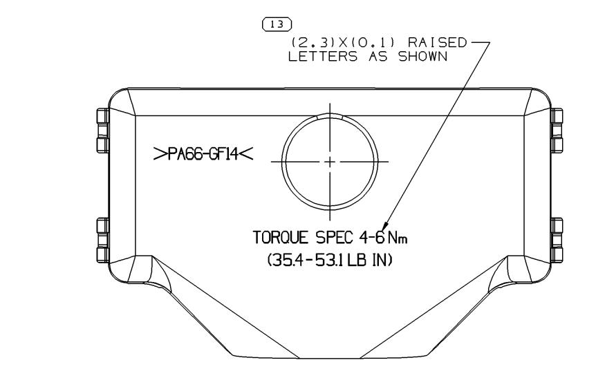
1. UNLESS OTHERWISE SPECIFIED AND/OR INDICATED: DIMENSIONS ARE TO FACE OF VIEW SHOWN AND AUTOMATICALLY ROUNDED BY COMPUTER FOR INSPECTION (SEE MATH MODEL FOR PRECISE DIMENSIONS). FOR ALL OTHER DIMENSIONS NOT SHOWN BUT REQUIRED FOR TOOL BUILD, SEE MATH MODEL FOR PRECISE TOOL PATH DATA. 2. MATERIAL RECYCLING CODE PER ISO 11469. (2.3)X(0.1) CHARACTERS AS SHOWN TO BE LOCATED ON ANY EXTERIOR SURFACE. 3. MATING PARTS: Connector asm 15488667 or equivalent (Wire dress towards cavities 1-8 and 33-40)
