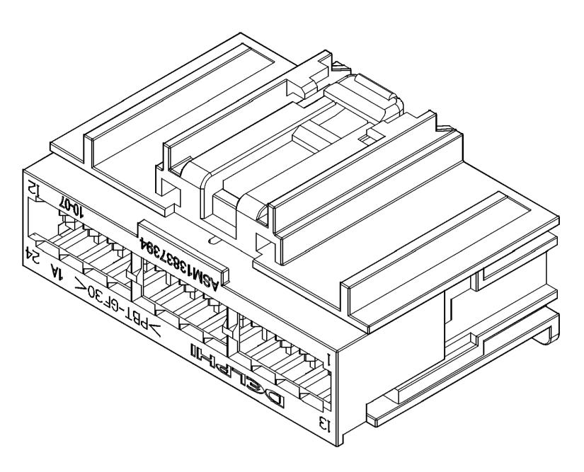
1. GENERAL TOLERANCE: UNLESS OTHERWISE SPECIFIED, ALL ANGULAR DIMENSIONS EXCEPT DRAFT: ±2° 0.3 MAXIMUM RADIUS ON EDGES AND FILLETS SHOWN AS SHARP. 2. UNLESS OTHERWISE SPECIFIED AND/OR INDICATED:
