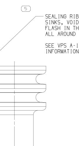
\_\_\_\_\_SEALING RIBS MUST BE FREE OF SINKS, VOIDS, KNIT LINES AND FLASHÍIN THEÍAREA SHOWN ALL AROUND PART. SEE VPS A-121 FOR ADDITIONAL INFORMATION.
