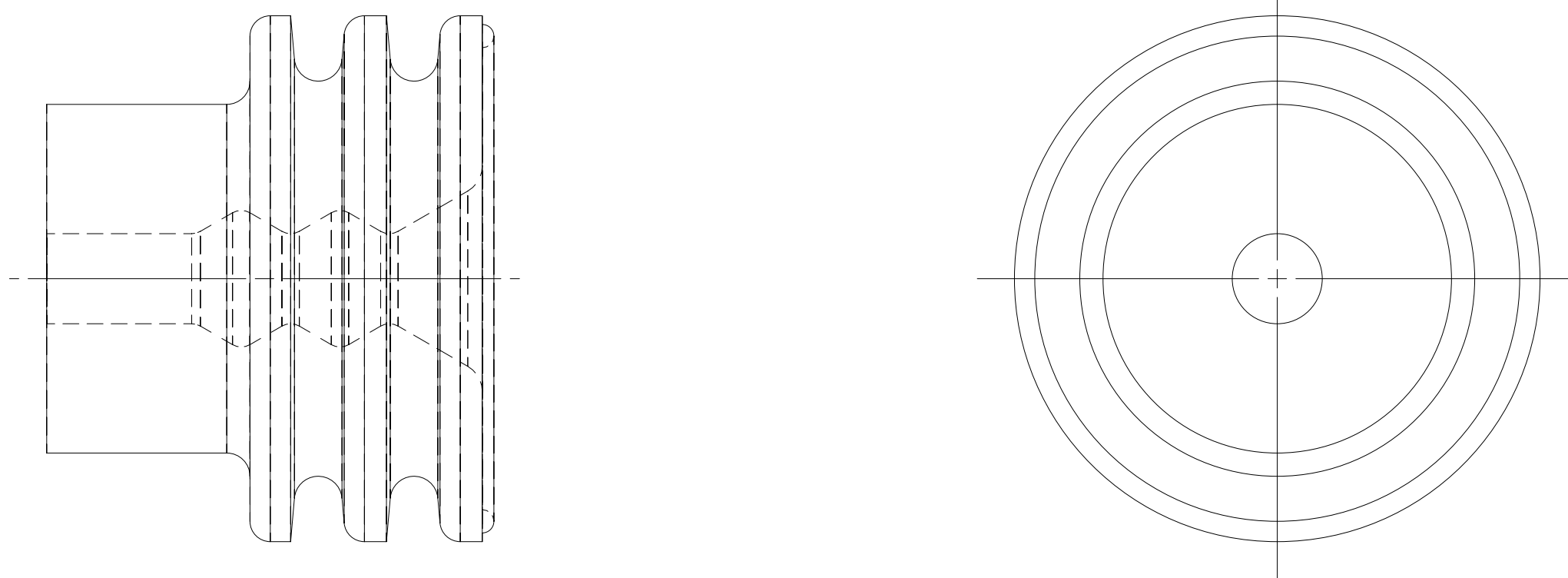
OPTIONAL CONSTRUCTION 2 THIS IS THE PREFERRED CONSTRUCTION FOR NEW TOOL BUILDS (ANTI-STICK RING)
