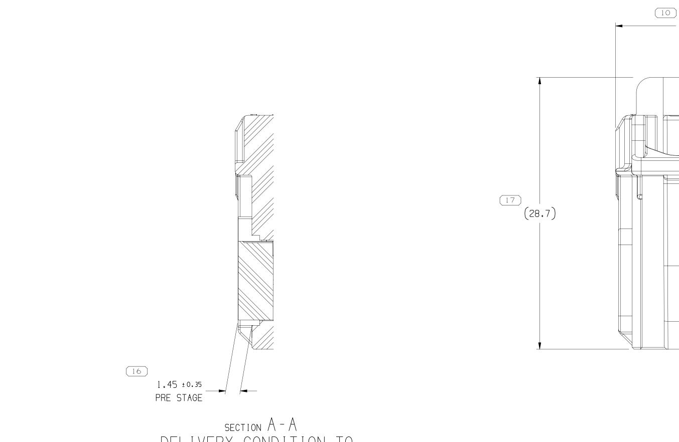
DELIVERY CONDITION TO WIRE ASSEMBLY PLANT FLS PRE-STAGED POSITION BEFORE TERMINALS
