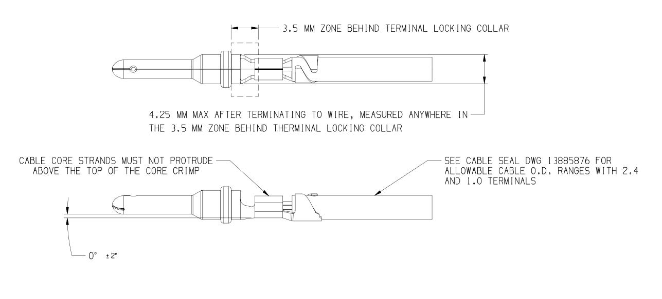
APTIV HES 2.4 TERMINAL - 13783284 OR EQUIVALENT WITH GOLD PLATED INTERFACE FOR POWER CIRCUITS. APTIV HES 1.0 TERMINAL - 13711545 OR EQUIVALENT WITH GOLD PLATED INTERFACE FOR SIGNAL CIRCUITS.
