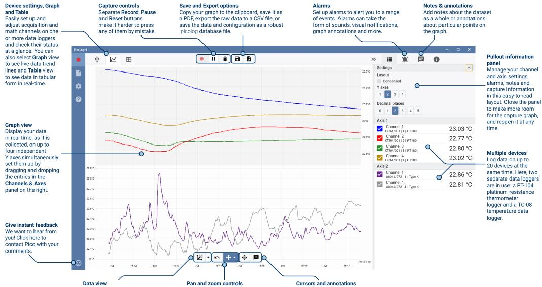
Display all the data collected so far or keep the graph scale the same and pan along as new samples appear.
