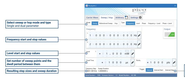
**Synchronize the sweep to a trigger** Internal clock, external input or software trigger sources. Trigger a sweep or trigger next point in sweep.
