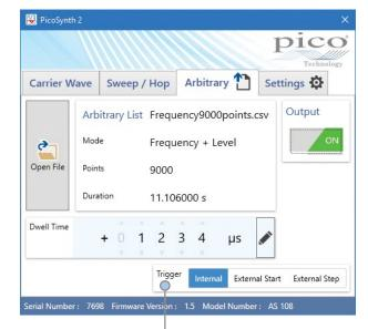
Trigger mode Internal: run continuously with the specified dwell time. External Start: run the whole file, with the specified dwell time, after each trigger event. External Step: generate one point for each trigger event (ignoring dwell time setting).
