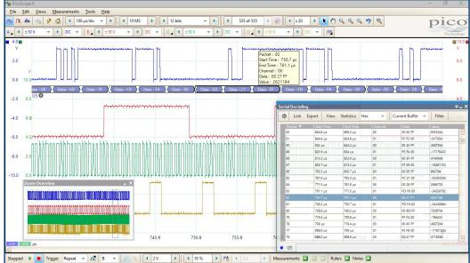
Table format shows a list of the decoded frames, including the data and all flags and identifiers. You can set up filtering conditions to display only the frames you are interested in or search for frames with specified properties.
