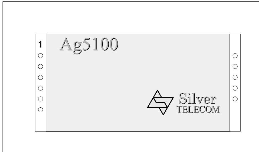
Figure 2: Ag5100 DIL Package Format (Top View)
