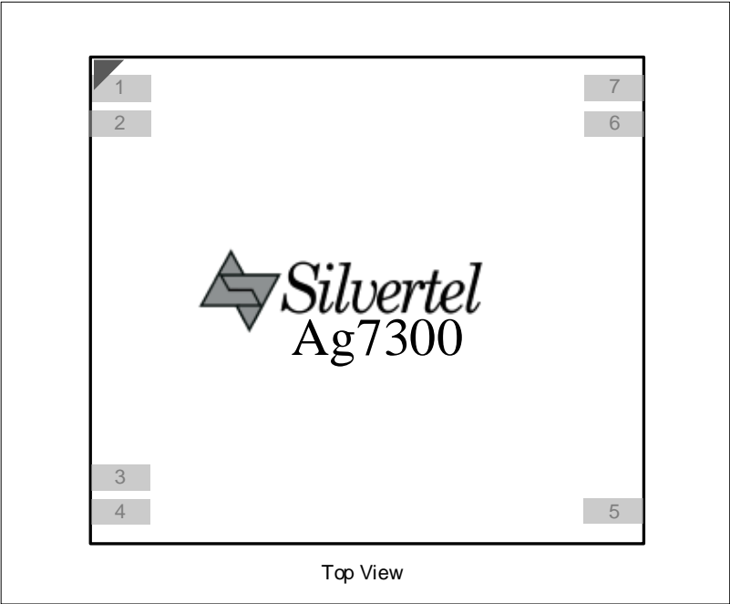
Figure 2: Ag7300 Package Format
