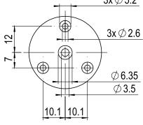
Board drillings Board thickness: 1.5-3.2 mm
