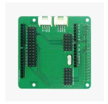
Raspberry Pi adapter for simpleRTK includes free basic technical support. Contact info@ardusimple.com for more information.
