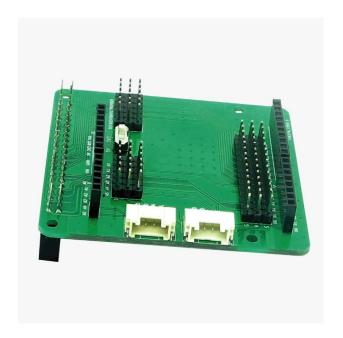
Raspberry Pi adapter for simpleRTK SKU is: AS-ADP-ARDUINO-TO-RPI-00
