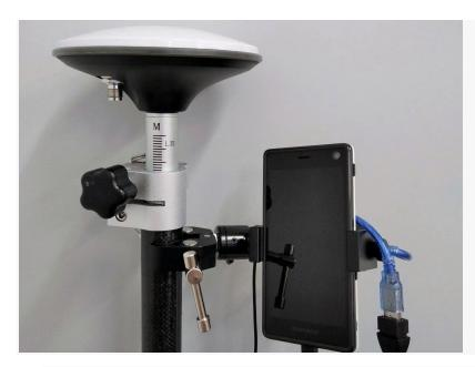
Finally, connect the TNC-K end of the cable to the Survey antenna and adjust the surveying pole to the convenient height.
