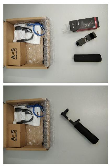
Mount the plastic case (simpleRTK2Blite + Bluetooth 2.0 within) to the smartphone holder. You will find the plastic case in a small box along with the helical antenna. To do this, fit the flat edge of the case with the outer part of the smartphone holder with the SMA connector facing up, and fasten it together with the velcro strap.
