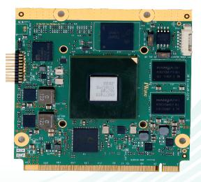
iWave's RZ/G1H based Qseven CPU module integrates Renesas RZ/G1H Quad core ARM Cortex A15 @1.4GHz & Quad core ARM Cortex A7 @ 780MHz CPU with rich set of features and IO peripherals. It integrates full HD hardware codecs, graphic acceleration, DDR3 RAM, eMMC Flash, Micro SD slot, USB HUB, HDMI transmitter and Gigabit Ethernet PHY. The SOM is ideally suitable for high performance video intensive and graphic rich applications.
