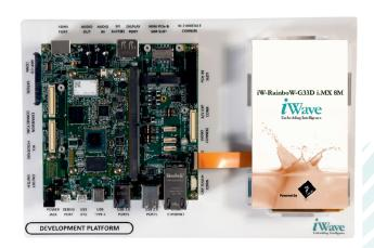
The i.MX 8M Quad/QuadLite/Dual SMARC Development platform combines the NXP's i.MX 8M Quad/QuadLite/Dual application processor based SMARC SOM and iWave's Generic SMARC Carrier Card to offer consumer, medical and industrial embedded computing & multimedia applications. The board is highly packed with all necessary onboard connectors to validate i.MX 8M Quad/QuadLite/Dual SoC features.
