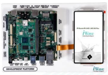
The i.MX 8M Plus SMARC Development Platform incorporates i.MX 8M Plus SoC based SMARC SOM and SMARC Carrier board for complete validation of i.MX 8M Plus SoC functionality. The Development board can be used for quick prototyping of various applications targeted by the i.MX 8M Plus Applications Processor. With the 120mmx120mm Nano ITX size, SMARC Carrier board is highly packed with all the necessary on-board connectors to validate the features of i.MX 8M Plus SMARC SOM.
