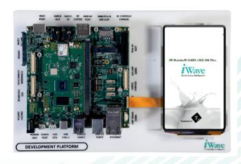
The i.MX 8M Plus SMARC Development Platform incorporates i.MX 8M Plus SoC based SMARC SOM and SMARC Carrier board for complete validation of i.MX 8M Plus SoC functionality. The Development board can be used for quick prototyping of various applications targeted by the i.MX 8M Plus Applications Processor. With the 120mmx120mm Nano ITX size, SMARC Carrier board is highly packed with all the necessary on-board connectors to validate the features of i.MX 8M Plus SMARC SOM.
