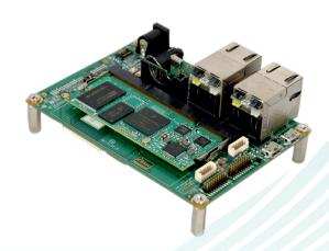
iWave's i.MX6ULL/ULZ development board incorporates i.MX6ULL/ULZ SODIMM SOM which is based on NXPs power efficient i.MX6ULL/ULZ ARM Cortex A7 processor and the carrier board with optional 4.3" resistive display kit. The development board can be used for quick prototyping of various applications targeted by the i.MX6ULL/ULZ processor. With the 100mm x 72mm Pico ITX size, and the kit is highly packed with all the necessary onboard connectors to validate the i.MX6ULL/ULZ CPU features.
