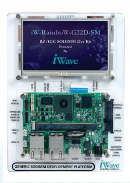
iWave's RZ/G1E SODIMM development kit incorporates RZ/G1E SODIMM SOM which is based on Renesas power efficient Dual core ARM Cortex A7 CPU cores operating @1GHz speed. The development board can be used for quick prototyping of various applications targeted by the RZ/G1E processor. With the 100mm x 72 mm Pico ITX size, the kit is highly packed with all the necessary on-board connectors to validate the RZ/G1E CPU features.
